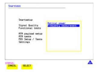
6 Press **SELECT** to display the frequency screen. Or press **CANCEL** to exit Smart Tests.
