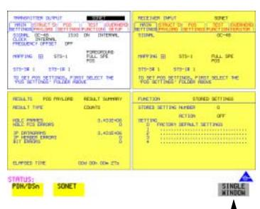
Press this key to select single window mode. The active window is then displayed (in this example TRANSMITTER OUTPUT would be displayed).
