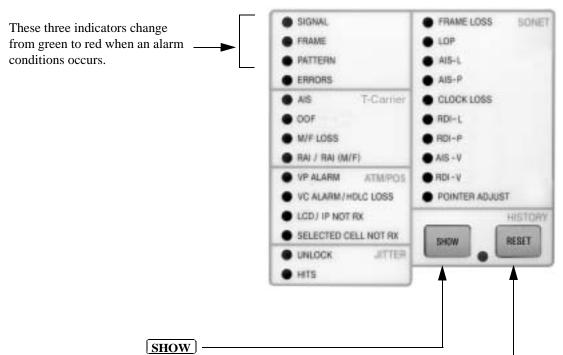
Press and hold this key to view the alarm history. When this key is released the status indicators return to displaying the current status.
