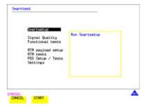
3 With Smartsetup highlighted, press **START** to auto-discover information about the receive signal. Or press **CANCEL** to exit Smart Tests.
